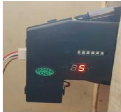
Fig.6. MultiCoin Acceptor showing the name of inserted coin.
